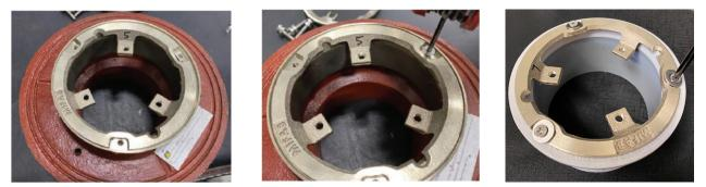
5 Attached the RTS5-1 collar to shank ring, align the 3 large set screws to destinated shank ring tapped holes. Alternatively tighten the set screws, few turns at a time.
