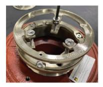
6 Attach the RTS5-1 strainer to shank ring. Then align the 3 peripheric chamfered holes with the peripheric small tapped screws of the shank ring. Secure the strainer in placeby using the 3 small set screws.
