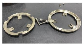
4 Assemble RTS5-1 shank ring on 5-1 Shank. Then align the 3 shank ring notches to the 3 tapped holes of 5-1 shank; secure shank ring in place with the 3 short set screws saved from 5-1. For JR SMITH and ZURN shanks use the provided washers to assemble the ring.
